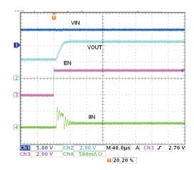
HT7936B V<sub>IN</sub>=4.5V, C<sub>IN</sub>=C<sub>OUT</sub>=2.2 $\mu$ F, C<sub>PUMP</sub>=0.22 $\mu$ F
