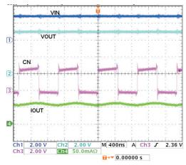
HT7936A V<sub>IN</sub>=2.8V,  $C_{\text{IN}}$ = $C_{\text{OUT}}$ =2.2 $\mu$ F,  $C_{\text{PUMP}}$ =0.22 $\mu$ F
