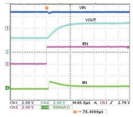
HT7936A V<sub>IN</sub>=2.8V,  $C_{\text{IN}}$ = $C_{\text{OUT}}$ =2.2 $\mu$ F,  $C_{\text{PUMP}}$ =0.22 $\mu$ F
