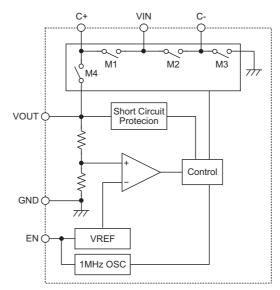
Note: During operation the following sequence occurs: 1. M1, M3 On / M2, M4 Off 2. M2, M4 On / M1, M3 Off
