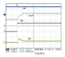
HT7936B  $V_{\text{IN}}$ =2.8V,  $C_{\text{IN}}$ = $C_{\text{OUT}}$ =2.2 $\mu$ F,  $C_{\text{PUMP}}$ =0.22 $\mu$ F
