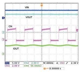
HT7936A V<sub>IN</sub>=5.0V,  $C_{\text{IN}}$ = $C_{\text{OUT}}$ =2.2 $\mu$ F,  $C_{\text{PUMP}}$ =0.22 $\mu$ F
